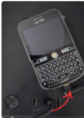
Figure 15: Device connected via USB ready for flashing
