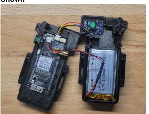
Connect the battery and insert both the battery and RTC into the case back as shown.
