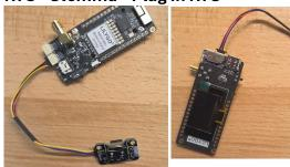
If you're using the Stemma verision of the RTC, simply plug it into the T3S3 as shown here.
