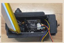
Be careful not to smash or pierce the battery! You may want to use electrical tape between components, where they may come in contact with one another or with the surface of the battery. The foil layer of the battery is conductive, so it can create shorts.
