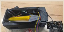
The Realtime Clock and GPS antenna (if equipped) can be inserted into the hollow area of the enclosure's top. I use a piece of electrical tape to temporarily hold them into place.
